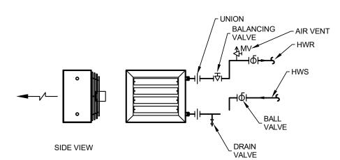
FAN COIL (4 PIPE), WITH GRISWOLDS DETAIL
